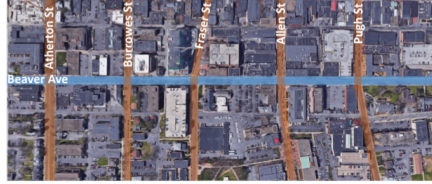
(b) Beaver Avenue in State College, Pennsylvania, USA: a 5-intersection arterial with unidirectional traffic on the arterial and bidirectional traffic on the side streets.
