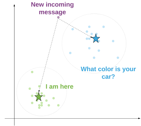
Figure 6: Illustration of the process of nearest neighbor classifier based on document embedding and cosine distance.
