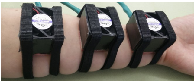
Figure 1. The Thermal Array Display (TAD) consists of three stimulator units, one positioned on the wrist, one under the elbow and the other between them.
