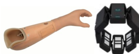
Figure 1. (Left) A myoelectric upper limb prosthesis – myo. (Right) The Thalmic Labs Myo Armband – Myoband.
