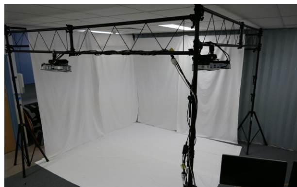
Figure 3. Hardware setup of Augmented Studio: 3x3x3m tracking volume with three sided projection screen and two projectors
