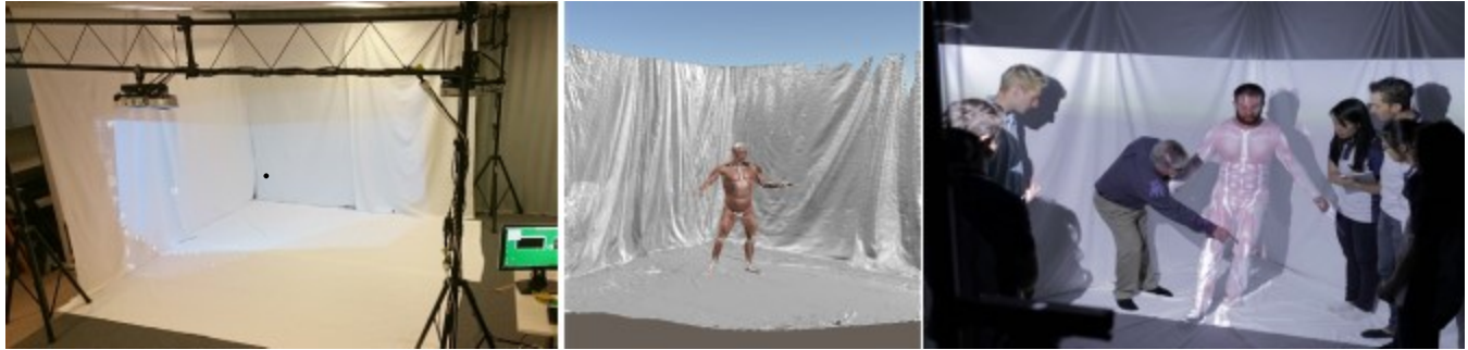
Figure 1. Augmented Studio setup: Left: the 3-sided stage, including scaffolding and 2 projectors with 2 Kinect sensors, set up in a physiotherapy practical classroom; Middle: the stage is captured virtually through projection mapping with a virtual anatomy model; Right: projected virtual anatomy model on a moving body for a physiotherapy practical class
