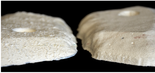
Figure 15. Comparison of surface texture in fabricated holds. (Left) Cast from a 3D printed hold with adhered sand. (Right) Cast from a porous foam hold.
