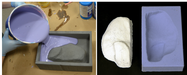
Figure 9. Molding & casting process. (Left) Silicone rubber poured over foam prototype to create the mold. The curing process requires 3-6 hours. (Right) Final cast climbing hold alongside its mold. Cast uses low viscosity resin which completes in under 5 minutes. The surface texture of the original foam is retained.
