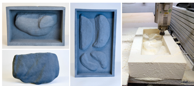
Figure 8. Foam holds carved with a CNC Router. Holds from “TATAN” route shown.
