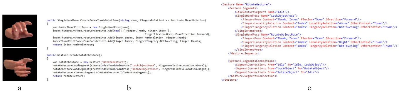
Figure 4. Gesture description in formal language: (a) A 'Rotate Right' gesture is composed of the two shown poses, starting with the index above the thumb, and ending with the index right of the thumb (from the user's perspective). (b) C# code that generates a 'Rotate Right' gesture object. The two comprising poses are defined using a single method 'CreateIndexThumbPointPose()' accepting the required index-to-thumb relation as input argument. 'Rotate Right' is then defined as a short sequence of the two poses. (c) 'Rotate Right' gesture defined in XAML format. The same propositions are applied, but without the C# syntax.
