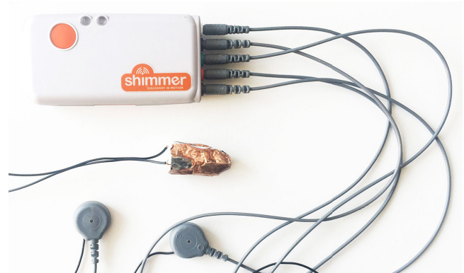
Figure 7. Shimmer3 ECG/EMG Bluetooth device, configured in EMG mode.
