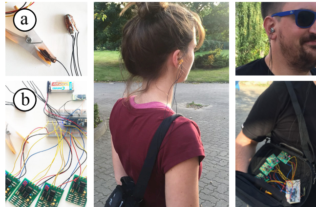
Figure 1. EarFS is a wearable electric field sensing device which enables to sense mobile facial-related gestures. It consists of a) an ear plug plus a reference electrode (a clothes peg that has to be attached to the ear lobe), and b) four sensing shields that are connected to an Arduino which runs on a 9V battery supply and transmits data via Bluetooth.
