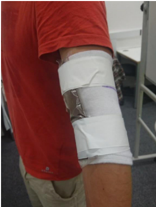
Figure 9. A patch attached to a participants arm. We used elbow supports to protect their arms from the vinyl tape used to secure the patches.
