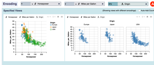
Figure 6. Wildcard shelf (A) allows users to consider alternative ways to encode origin (by using color or by faceting).
