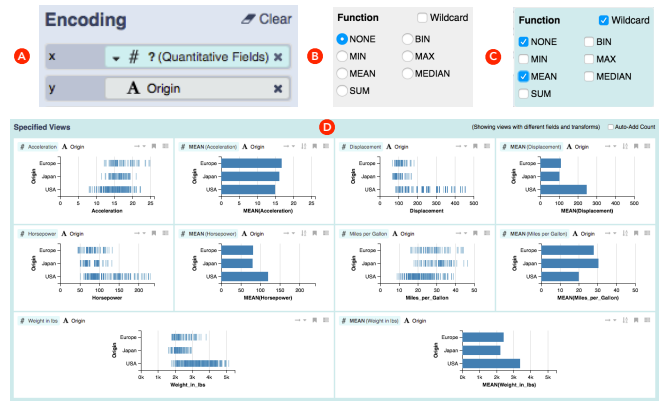
Figure 5. Mapping a quantitative field wildcard to x and origin to y (A) produces a gallery of plots. A wildcard function enumerates no function ( none ) and mean (B-C), generating strip plots of raw values and bar charts of mean values (D). The ? in (A) denotes the wildcard function.
