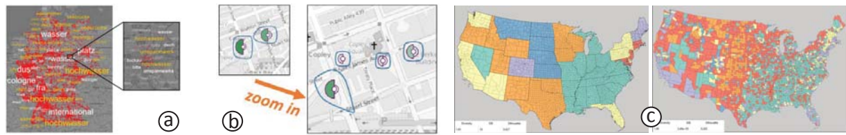
Figure 2. Examples of multi-scale clustering: (a) Keywords are aggregated and displayed on the map (Tag Map). Zooming into the map shows lower-level sub-events [34]; (b) Spatial clusters are visualized at consecutive zoom levels. Large clusters at a higher zoom level split into multiple small ones at a lower level [42]; (c) Clustering results of demographic statistics under different geographical resolutions (left: state level, right: county level) [43].
