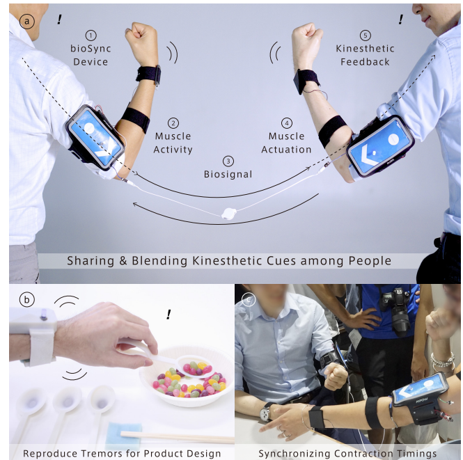
Figure 1. (a) Synchronizing and combining muscle activities among people (b) Reproducing kinesthetic experience of Parkinson's impairment for use in supporting product design (c) Participants express surprise when the muscle activity is jacked in by the demonstrator
