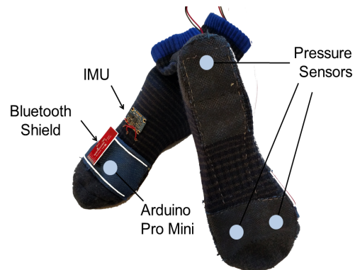
Figure 1: The wearable components of SoPhy : Each sock consists of three pressure sensors and one IMU.
