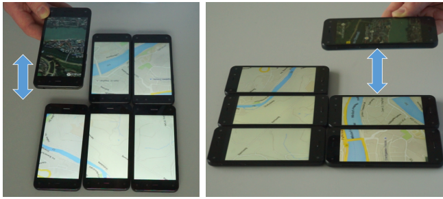
Figure 3: Map applications multiple map layers can be browsed by changing the height of individual devices.
