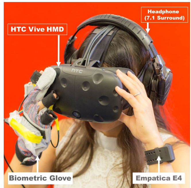
Figure 1. Participants were asked to stand during the gameplay sessions. They were wearing HTC Vive HMD and two different heart-rate sensors - Empatica E4 and Biometric Glove with Arduino sensors. They were also wearing a Logitech noise canceling headphone to hear the sounds of the game.
