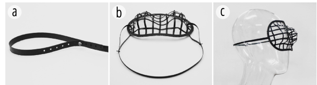
Figure 9. Belt clasp structure: (a) the belt, (b and c) an application: a blinder.
