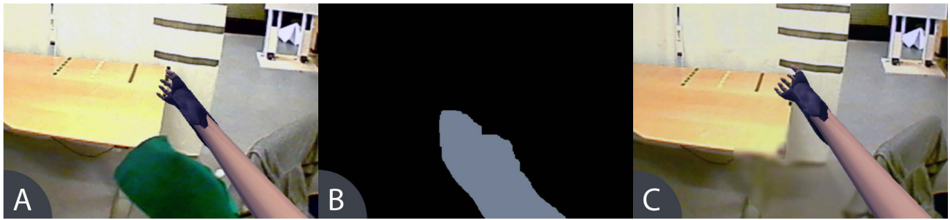
Figure 3: (A) Hand in green sleeve, (B) binary mask after chroma keying, (C) Memory Inpainting .
