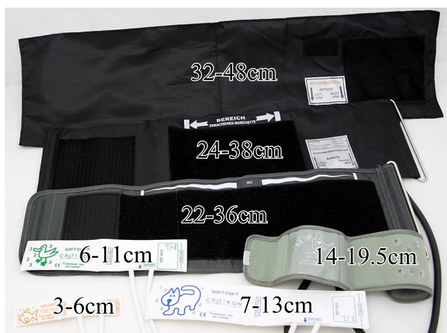
Figure 3. We used a wide range of blood pressure cuff sizes to test our system on several body locations. The smaller cuffs can be wrapped around single or multiple fingers, the 14-19.5 cm cuff fits around a wrist, while the larger cuffs fit around upper arms and legs.
