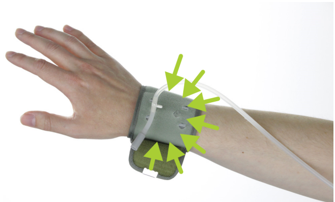
Figure 1. Compression feedback ranges from very subtle to very intense and is well suited for intimate communication and background feedback. We use pneumatic actuation and inflatable straps to create stimuli.
