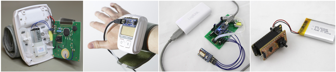
Figure 4. We built several compression feedback controller prototypes. They all reuse parts from off-the-shelf blood pressure monitors (shown in leftmost image). We only keep the sensor and valves at the wrist for our first prototype (second image), but move the pump to reduce its influence on the sensation. The second prototype (third image) is designed for mobile evaluation, fits into a pouch, and is controlled from a phone via a Bluetooth module. The third prototype (last image) miniaturizes this setup for even better mobility.
