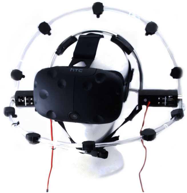
Figure 1. The VaiR Prototype worn in combination with a HTC Vive head mounted display. Fixed to frame mounted onto the Vive's straps are two bows. These bows are moved by two separate motors, allowing both bows to each rotate 135°. Fixes on each bow are five nozzles (each 36° apart), where the air streams come out. Several nozzles can be used at the same time. Due to the modular design, nozzles can be moved along the bows and changed as needed. That way, angle and dispersion of the air streams can be customized. VaiR is so designed that a container of pressurized air, valves, power source and an arduino controller can be worn as a backpack.
