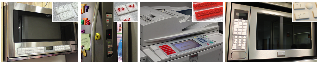
Figure 1. Facade is a crowdsourced fabrication pipeline that enables blind people to make flat physical interfaces accessible by independently producing a 3D-printed overlay of tactile buttons. From left to right, we demonstrate example applications including microwave, refrigerator door, copier, and another microwave. Insets show close views of individual embossed buttons.
