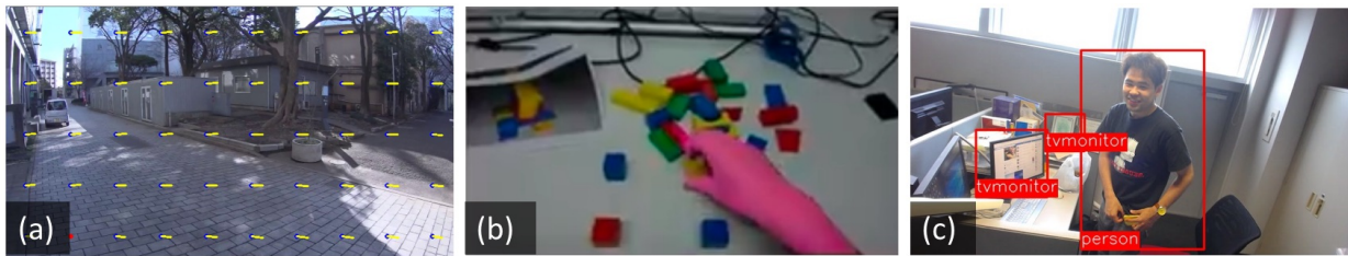
Figure 3. Extracting egocentric cues from first-person videos. (a) Sparse optical flows for movement and stop cues; (b) Pixel-level hand detection for a hand cue; (c) Object detection for a person cue.
