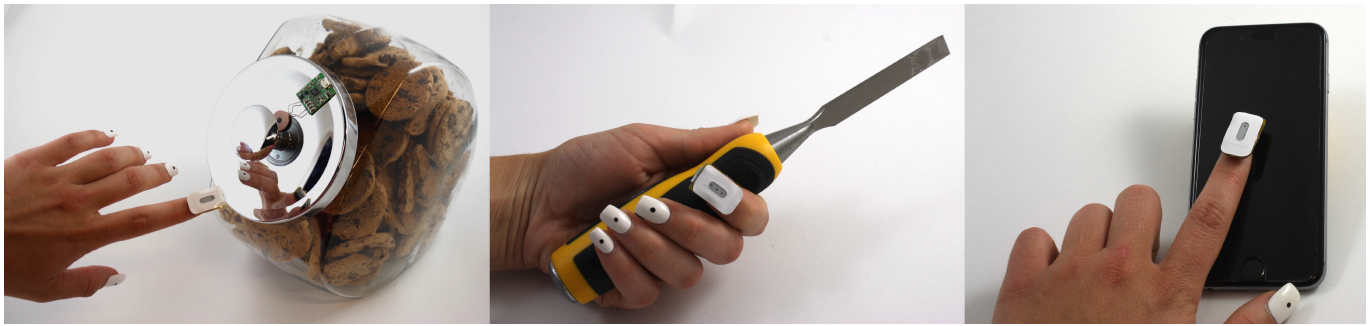
Figure 3. Left: Credits and Usage scenario demonstrated with an AlterNail enabled cookie jar. When the user opens the cookie jar, a new dot is added to their AlterNail display. Middle: Object Status scenario demonstrated with an AlterNail enabled chisel. As displayed by the AlterNail, this tool has been used three times today. Right: AlterNail updated through NFC from a smartphone. The user can discreetly check that they have one new email without unlocking and looking at their phone.
