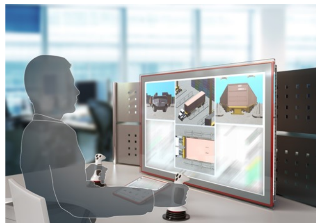
Figure 2. Concept illustration of the ROS system with the four-view setup in the main display
