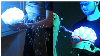
Figure 16: The soap in action, controlled by ultrasonic distance sensor (highlighted on the right).
