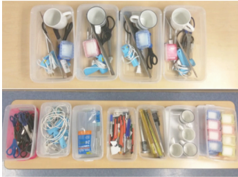
Figure 1: Traditional kit-based arrangement of tools and materials (top) versus a workbench-based arrangement of tools and materials (bottom). Traditional kits can be assembled and disseminated to student groups, whereas workbench arrangements require students to come and select what they want to use. Each can be suitable depending on the activity and are easy for instructors to prepare.
