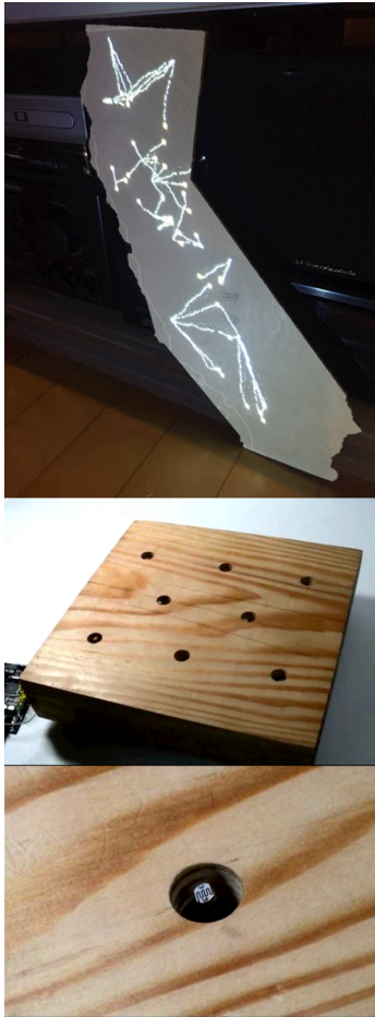
Figure 3: A Prototype of California Drought Impact v2 with a digital projection image on a wooden sculpture and new wooden interface with photocell sensors.
