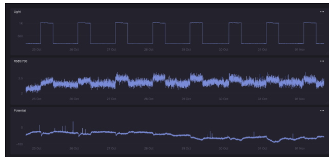
Figure 5: 8 day long experiment with a tomato plant measuring variation potential and fluorescence spectra changes (R685-730nm) in relationship to a 8h blue and red light cycle
