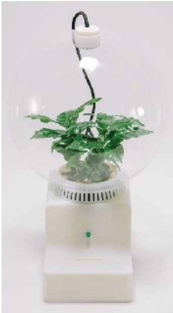
Figure 1: Project Florence Base piece containing a living plant instrumented with a variety of sensors to measure temperature, soil moisture and humidity. Additionally, the LED at the top displays Red or Blue light on to the plant depending on the user's sentiment. The plant will print out a response via a mini printer installed below the plant.
