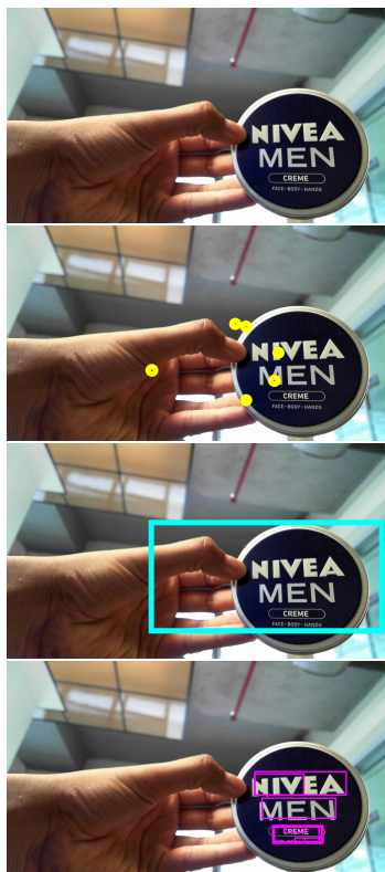
Figure 3: Example text-recognition on object. (a) Raw frame captured (b) Approximate finger and palm positions are calculated, with correspondence mapping to camera frame (in yellow). (c) ROI estimation and cropping (in cyan). (d) Extremal-Regions classification on the ROI (in magenta). The final detection in the image is "NIVEA MEN CREME FACE BODY HANDS".
