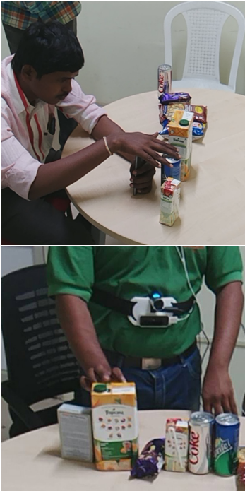
Figure 2: (a) VIP using TapTapSee, a mobile app for object detection. He uses his right hand as a “ruler” to ensure the correct distance between the phone and the object. (b) Close-up shot of VIP using FReAD to identify objects in a controlled testing environment. The device naturally allows the user to explore the objects with their hands without interrupting the detection.
