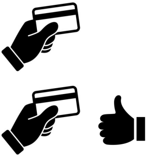
Figure 5: Programmed gestural metaphors. (a) A generic grasp yields a computational object detection that includes text and color. (b) A thumbs-up gesture after the object has been grasped triggers a crowd-labeling request.
