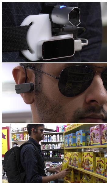
Figure 1: (a) View of FReAD's belt-style wearable system, worn around the user's waist. The height is adjustable, but generally sits at the waist or belly. (b) View of the bluetooth headset. (c) View of user shopping while wearing the FReAD belt.
