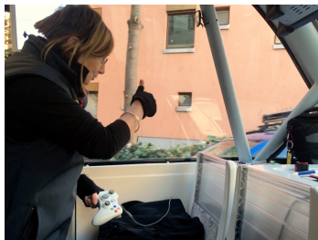
Figure 3: An onboard attendant monitors and manages AV operations at all times. If necessary they can control its steering, acceleration and braking using a reconfigured Xbox controller in real-time traffic situations.
