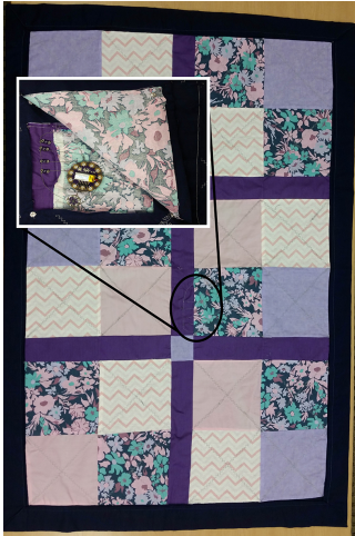
Figure 1: Research team's demonstration quilt, which included a LilyPad Arduino with conductive thread, LEDs, and an accelerometer. The cutout is the quilt's back flap hiding the electronics.
