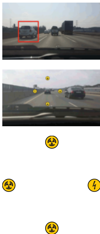
Figure 4: The first and second pictures show captured scenes from the prototype we have developed with MATLAB (Mathworks, Natick, MA). The last picture shows the example icons for UFOV interface. The lightening sign was a target icon of which drivers had to find the direction.
