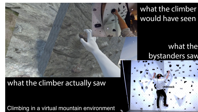
Figure 1: Visualization of the virtual reality climbing system. The integrated field camera of the HTC Vive was used to capture the view that the climber would have seen.
