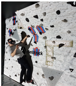
Figure 6: Using a projector, the virtual environment is projected back on the physical climbing wall to reflect the interactions of the player in the VE.
