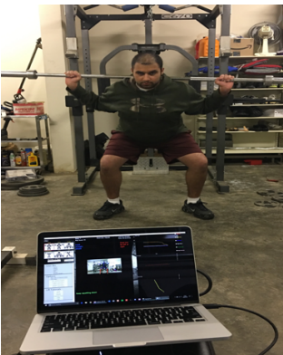
Figure 2: Our system warns a user that the bar is no longer level during a squat exercise. This error is stored so that a user may review their lift at their convenience. Our system aims to be implemented alongside a screen so the user may see the feedback that is being processed real-time and correct their form.
