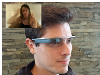
Figure 2: Informal testing involved use of Google Glass. Note that video projection of ASL or captions is onto the Glass display in the upper right for users. ©RIT.
