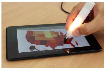
Figure 8: Additional information of a visualization are displayed on a LED module.
