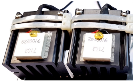
Figure 4: Peltier thermal stimulators (2 x 2cm 2 ) used in the lab study, with heatsinks.
