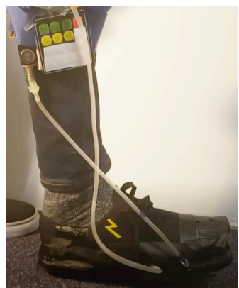
Figure 2: (top) The two-part inflatable layer allows independent ball and heel elevation; (middle) the prototype uses leg mounted controls to allows the user to personalise their desired support; (bottom) a user wearing the Inflashoe.
