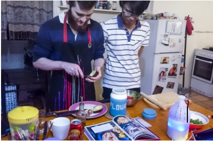
Figure 3. The performance apron and talking bottle in action: when the user presses a button on the apron the bottle will record the ambient sounds together with any messages or conversations. The recordings are sent to a corresponding device where they can be replayed. The bottle (bottom right) glows when a message is present.
