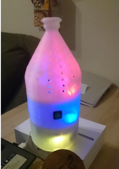
Figure 4. The Talking bottle glows in different colours to signal the availability of voice messages or that someone is cooking in the remote kitchen.
