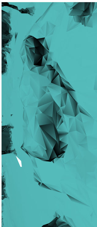
Figure 1: 3D mesh of a mannequin on a table as generated by HoloLens' spatial-mapping algorithm and rendered through its web interface.
