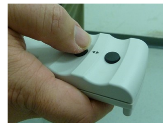
Figure 5: Two button remote control (with perceivable pressure point for each button) connected by cable.
