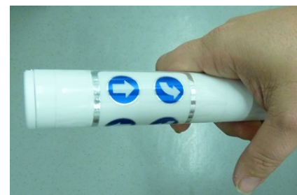
Figure 7: Buttons (membrane foil) integrated in a grip bar.
