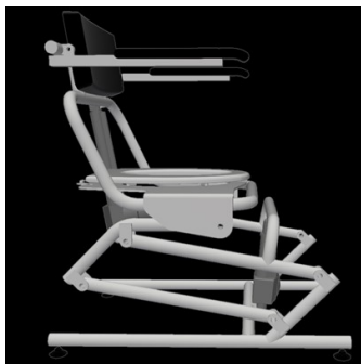
Figure 1: Height and tilt adjustable base module intended to be put on top of existing toilet bowl. Drawing: Santis Kft.
