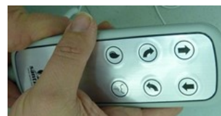
Figure 6: Six button remote control (membrane keyboard).
