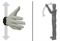
Figure 8: Vertical shaking gesture. (L) Watch display faces wall; fast arm movement in vertical direction. (R) Fast arm movement in vertical direction with right arm.
