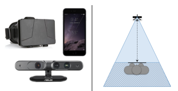
Figure 3: 3D camera setup: Asus Xtion Pro Live 3D camera and VR viewer fixing iPhone 6Plus (left). Viewing angle of camera limits user's movement ability (right).
