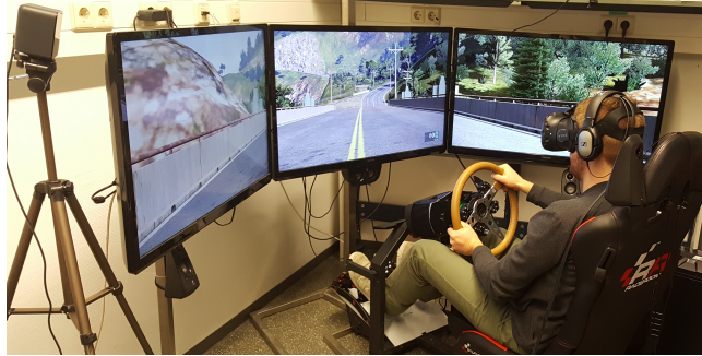
Figure 1: Experimental setup: Participants saw the game [21] either on the flat screens in front of them (traffic scene and a speedometer) or via a VR HMD (see in-cockpit scene in Figure 2).
