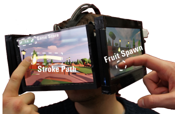
Figure 3: A closeup of two users interacting with FaceDisplay. Highlighted are the slicing path the HMD user created and the spawn location of the next fruit.
