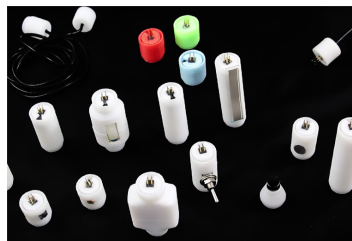
Figure 1: Set of modules composing the pen, including sensors and displays.
