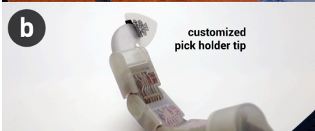
Figure 6. the tip module can be designed to perform a variety of operations, such as holding a pick (b), in turn allowing a remote user to help with a range of physical tasks such as teaching how to play the guitar
