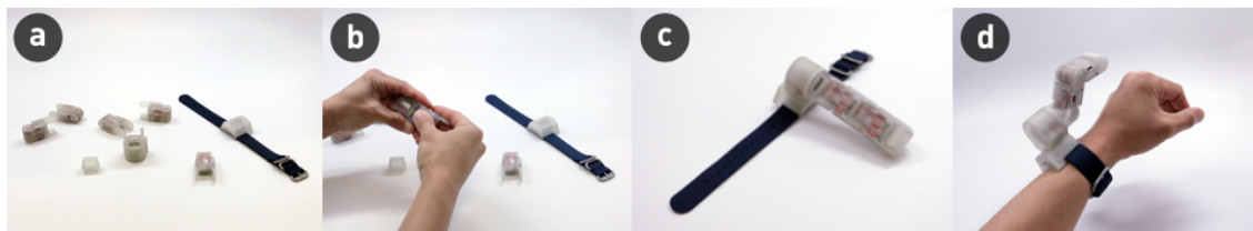
Figure 1. a) modules for robot assembly b) the modules are connected by a single clasp action c) an assembled robot connected to the wrist attachment module d) the robot in action, worn on a user's wrist
