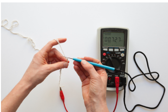
Figure 4 Using a connectable crochet hook to crochet a textile stretch sensor.
