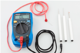
Figure 5 A multimeter with custom test leads. The red cord has a pin at the end, the black cord connects to needlecraft tools.
