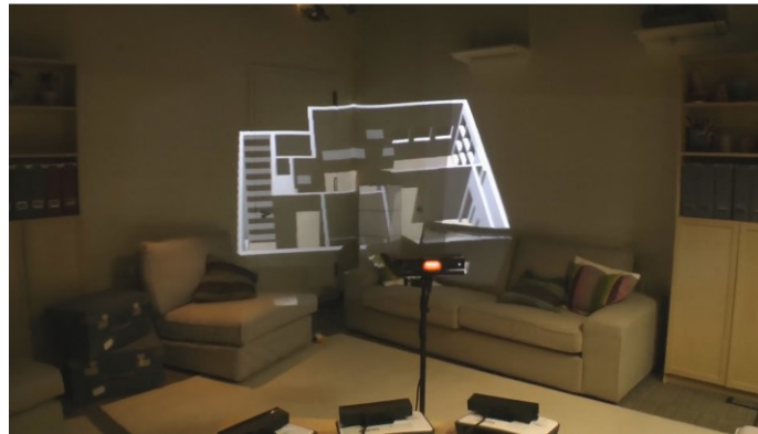
Figure 3. A simple RoomAlive installation demonstrates view-dependent rendering of a 3D object. Three projectors and three cameras are used to projection map the room, while a fourth camera (center) is used to track the head position of the viewer. The 3D model of an apartment floor plan appears as a 3D object hovering between the viewer and the walls.
