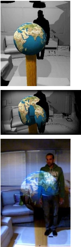
Figure 1. Dynamic projection mapping can be used to project onto moving bodies, for example. Top: desired view; middle: projected graphics; bottom: resulting view.
