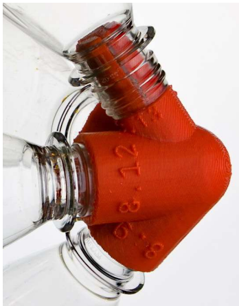
Figure 2: TrussFab generates 3D printed hubs. Users assemble them following embossed IDs.
