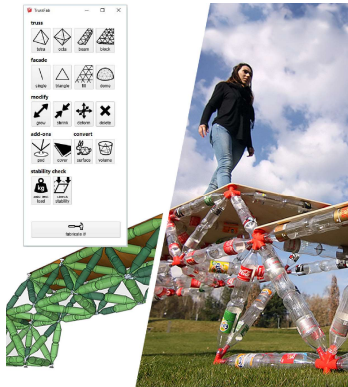
Figure 1: TrussFab allows users to fabricate large structures sturdy enough to carry human weight. TrussFab uses bottles as beams to form trusses .
