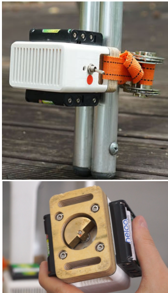
Figure 1: Attachable modules with an eccentric rotating mass vibration motor.
