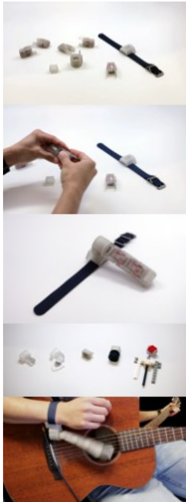
Figure 2: (from top to bottom) 1) designed modular components, 2) assembly of the modules, 3) assembled robotic configuration 4) mounted on the attachment module, 5) customized end-effectors, 6) a robotic configuration in action.
